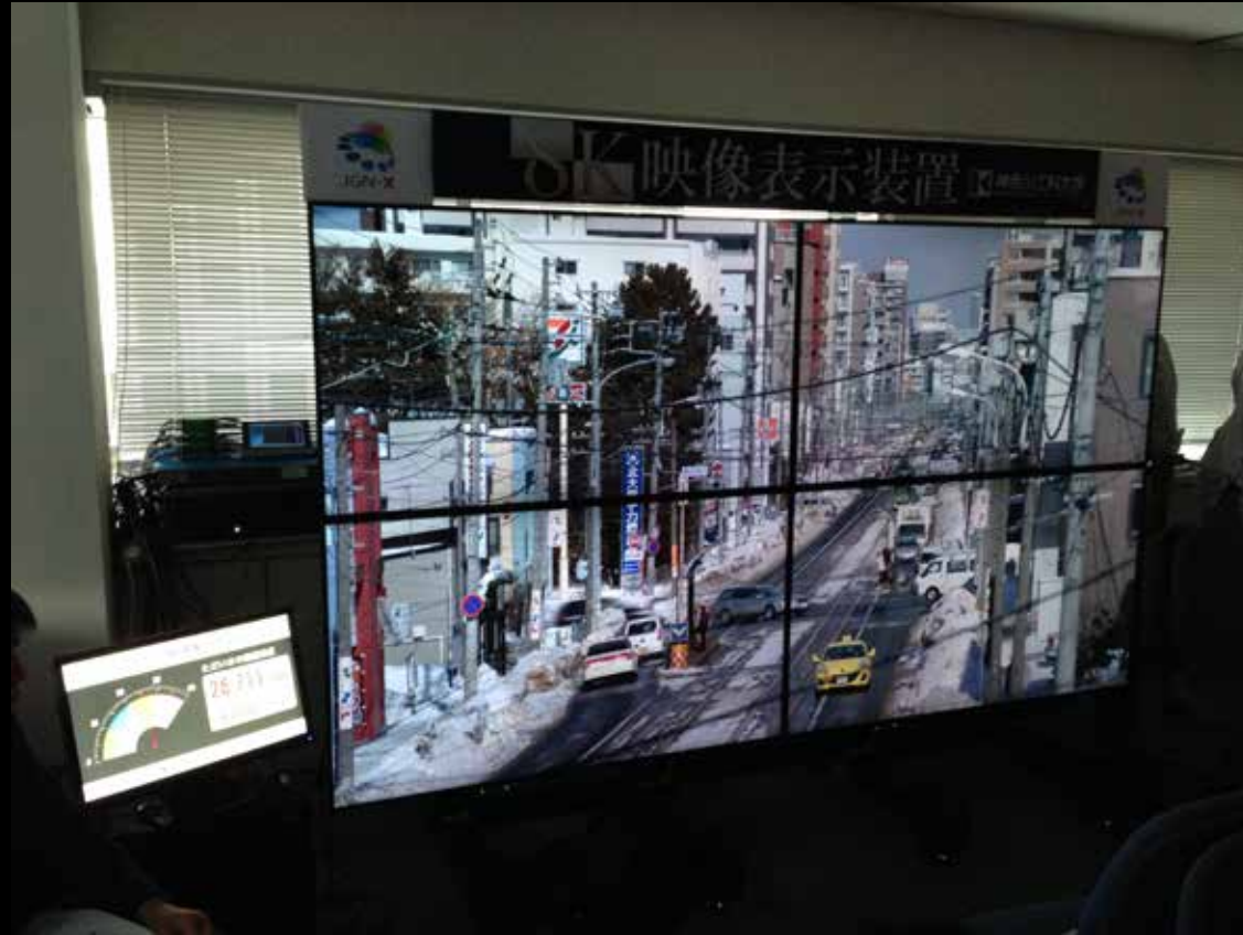
8K real-time streaming video from XMS@Osaka on 8K monitor made from four 4K LCDs
