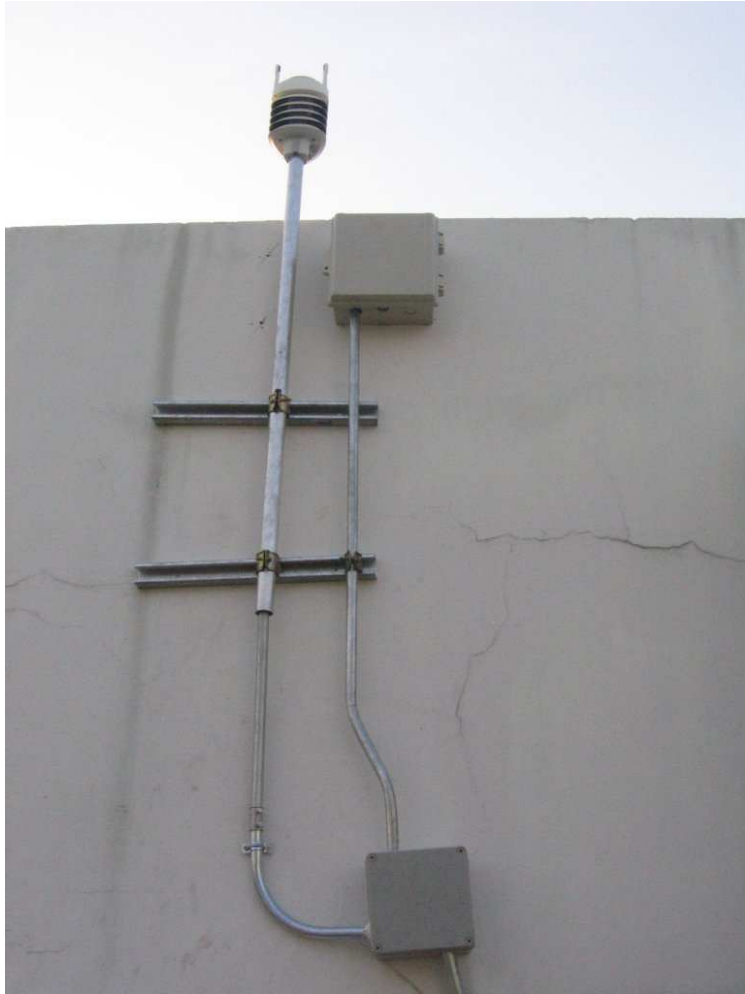
Weather Sensor (WXT510) in Kasetsart University
