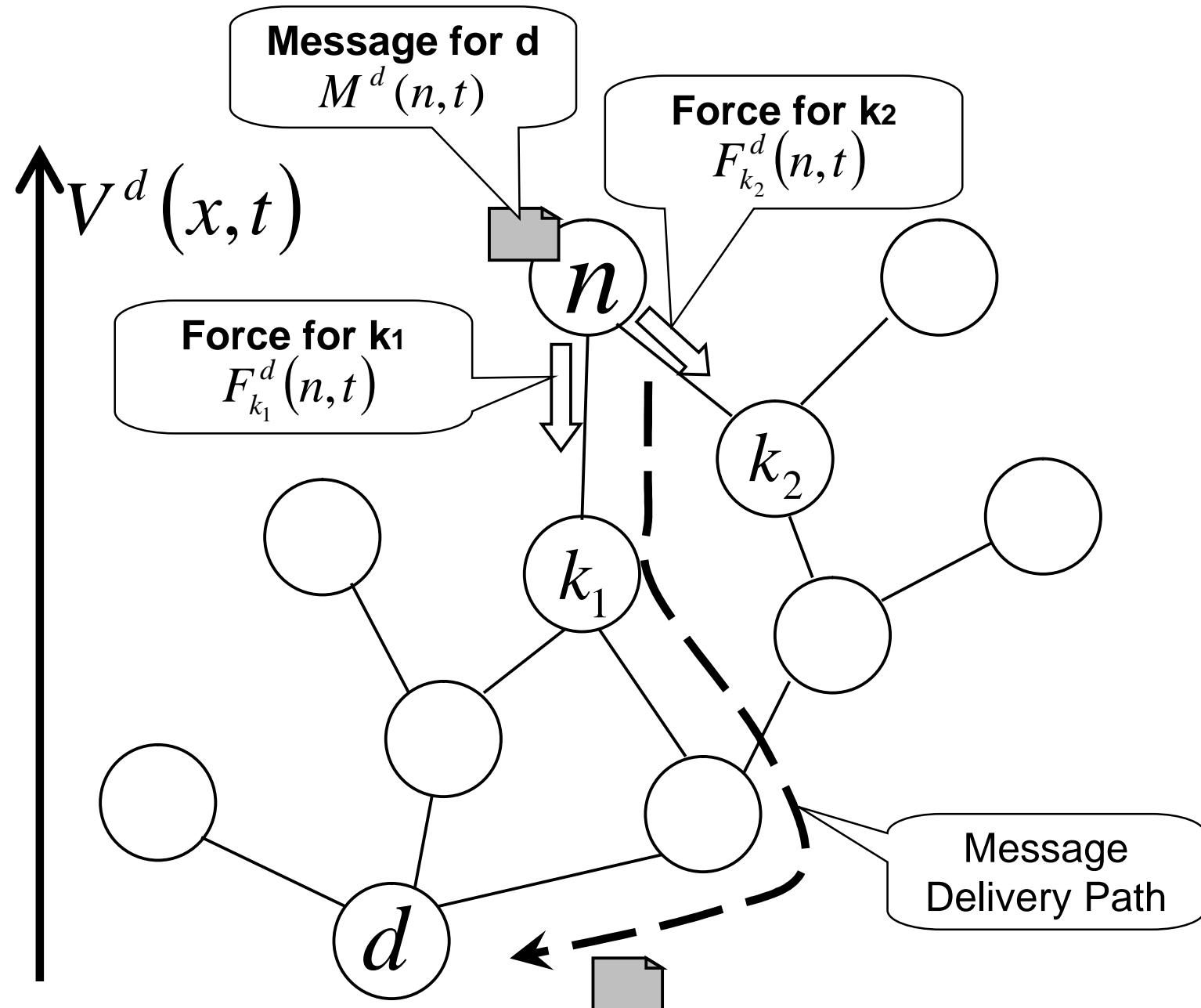
$$\{F_{k_1}^d(n, t) > F_{k_2}^d(n, t)\} \wedge \{F_{k_1}^d(n, t) > \alpha\} \rightarrow \text{nexthop}^d(n, t) = k_1$$
